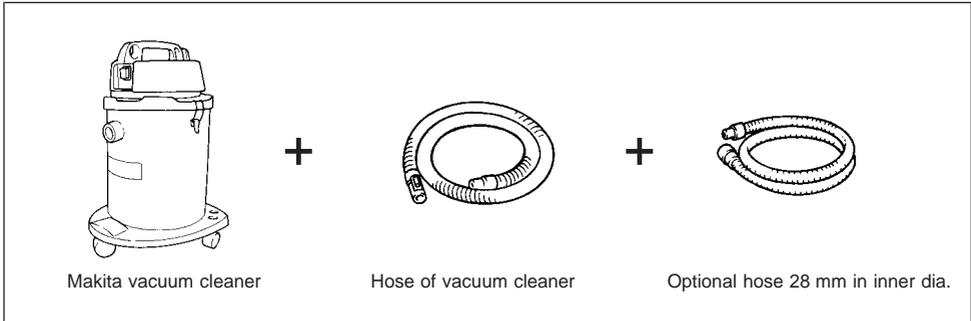
When connecting to Makita dust collector (Model 420), the optional hose is not necessary. You can connect the belt sander directly to the hose of the dust collector.
